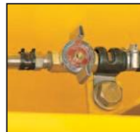
Fuel Drain Valve
